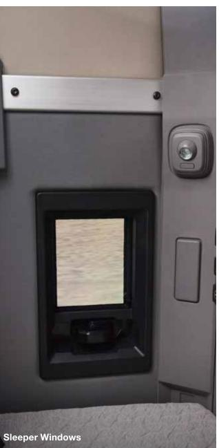
Sleeper windows feature self-contained bug screen and built-in shades that block 100% of light. The screened windows tilt out to let air in and keep
